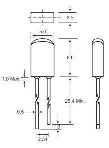
Unit: mm (inches) Tolerance: ± 0.25mm (.010") max.
