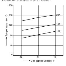
1-(2). Coil temperature rise (at 85°C 185°F) Sample: CR2-12V, 5pcs Contact carrying current: 10A, 15A
